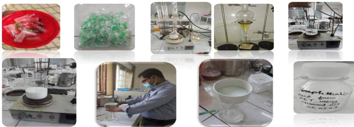
**Picture 01: Recovery of terephthalic acid from waste PET flakes by alkaline hydrolysis.**
