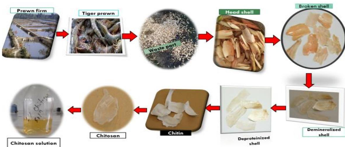
**Figure 1:** Production and activation of chitosan from shrimp/prawn shell waste during laboratory experimental session (photographic representation along with flow diagram).
