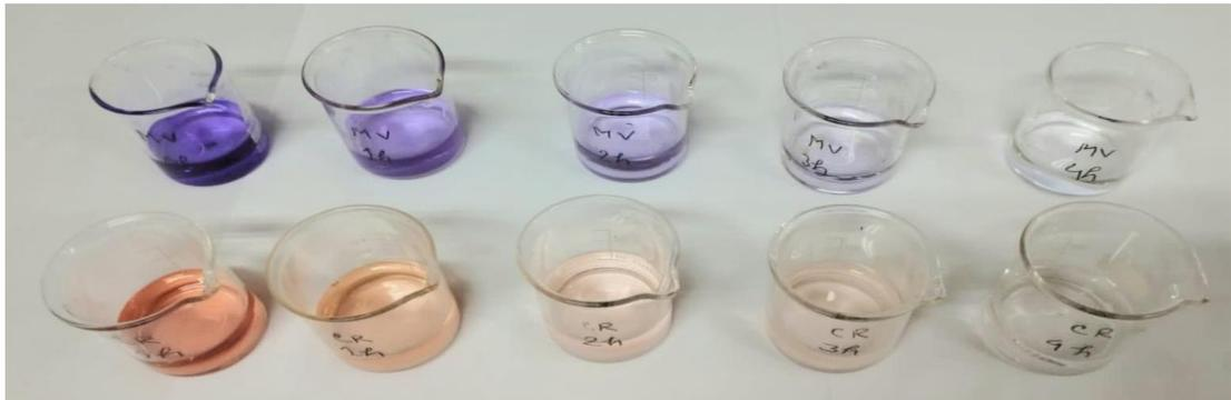
Figure: Methyl violet (MV) and Congo red (CR) dye degradation using HAp
