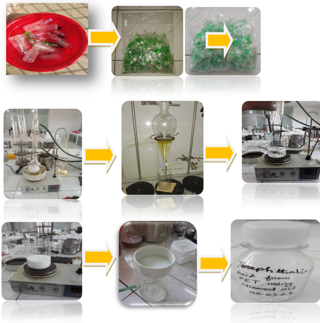
Figure: Terephthalic acid isolation flow chart from waste PET bottle.
